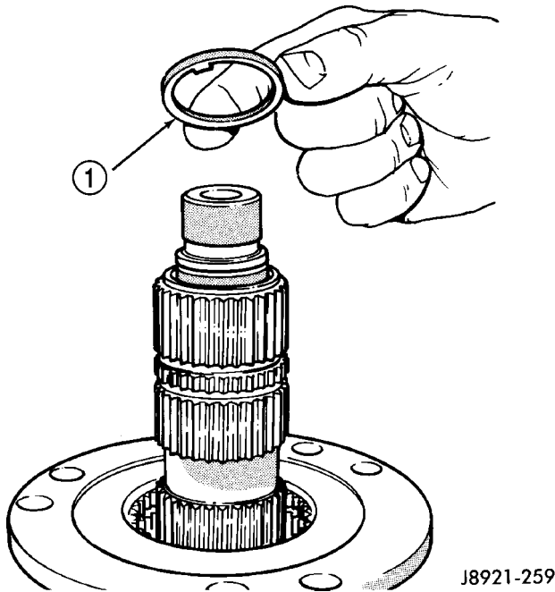
Fig. 28 Clutch Shaft Thrust Ring Removal
