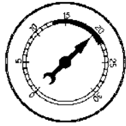
NORMAL READING RANGE AT IDLE
