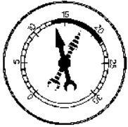
STICKING VALVE AT IDLE
