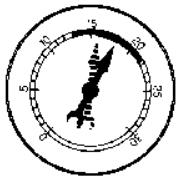
POOR VALVE SEATING AT IDLE
