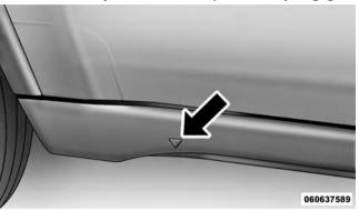
Lift Point Symbol On Sill Molding
