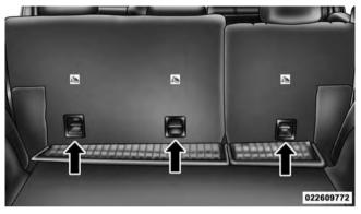
Top Tether Strap Anchorage (Located on Seatback)
