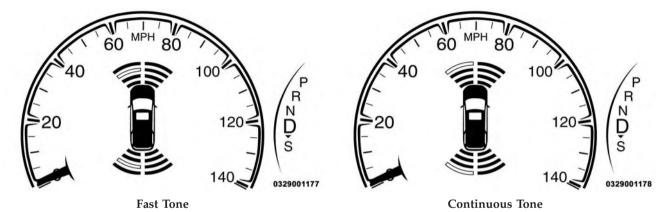
The vehicle is close to the obstacle when the EVIC display shows one flashing arc and sounds a continuous tone. The following chart shows the warning alert operation when the system is detecting an obstacle:
