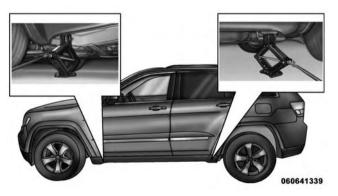
4. For the front axle, place the jack on the body flange just behind the front tire as indicated by the triangular lift point symbol on the sill molding. Do not raise the vehicle until you are sure the jack is fully engaged.
