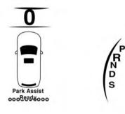
The system will indicate a detected obstacle by showing a single arc in the left and/or right rear regions based on the object's distance and location relative to the vehicle.
