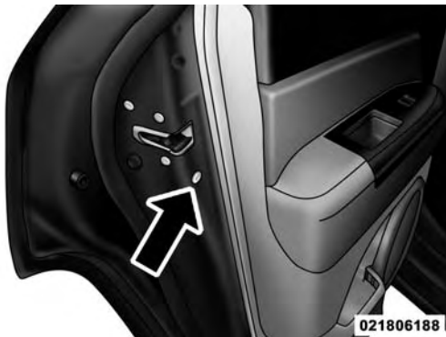
Child-Protection Door Lock Location
